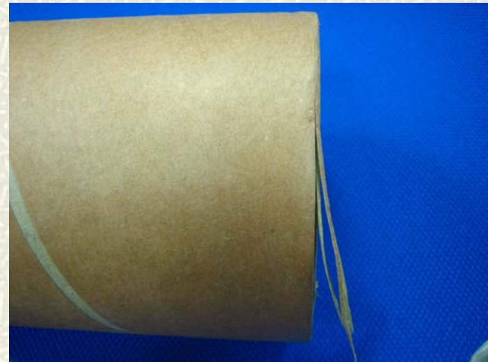
Cut-Edge has 1mm error(leading)
